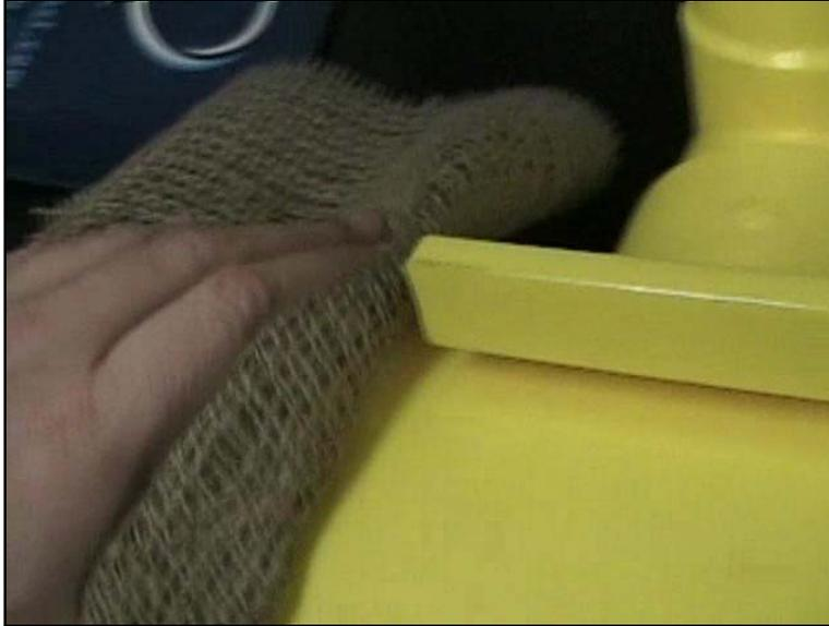
**Figure 5. Static Suppressor Test: Soapy burlap application.**
