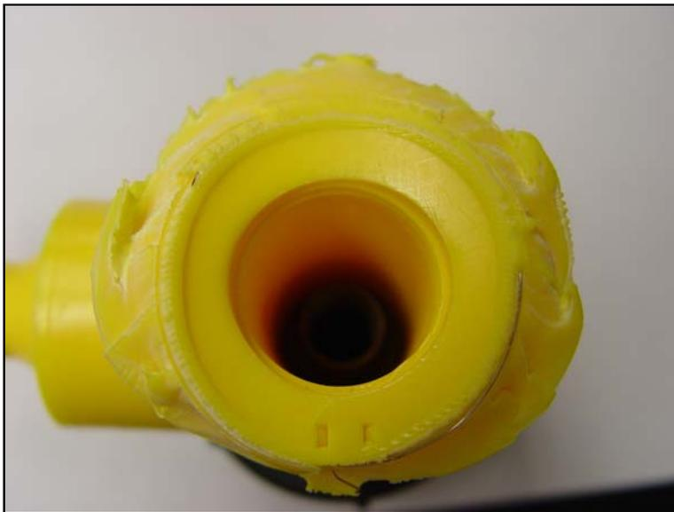
**Figure 8. Impact Test: Close-up look at tee. Note how the weight completely tore the stem off of the central gas electro-fusion saddle tee. This is consistent with properly fused PE material (plastic material itself failed, not the fusion).**
