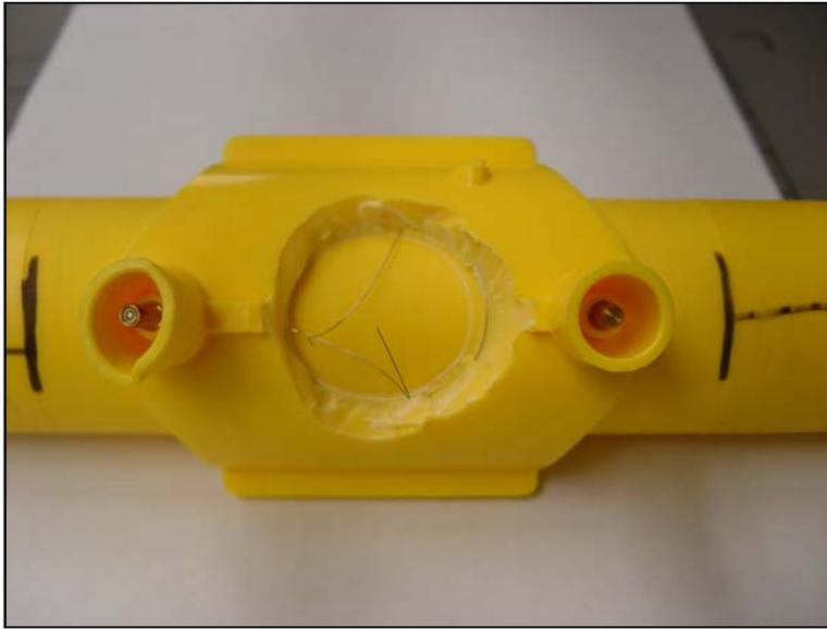
**Figure 7. Impact Test on electro-fused saddle tee to ASTM F905.**
