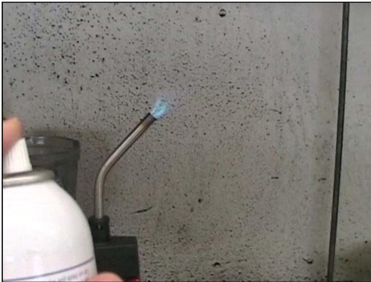
**Figure 6. Flammability Test. Note that the flame does not increase when sprayed with IGT static suppressor.**
