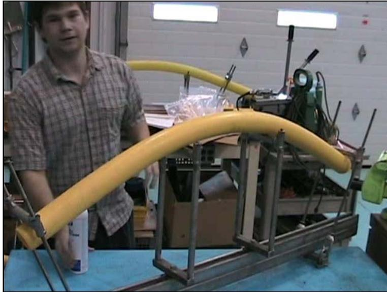
**Figure 1. ASTM D543 Chemical Resistance: Pipe Bend Test Fixture set at 10 times the outside diameter. Sprayed pipes were compared to control pipes of same 2" UPONOR MDPE 2406 vintage.**
