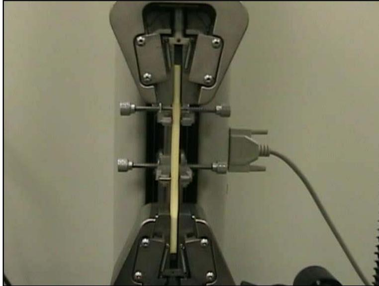
**Figure 3. ASTM D638 Tensile Test: MTS Machine used for testing.**
