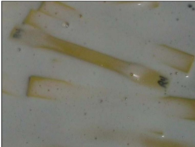
**Figure 2. IGT spray bath with dye cuts to compare the modulus, and yield strength to control samples from the same pipe.**
